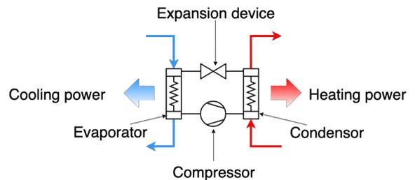
Figure 3. Operating principle of the simultaneous heating and cooling heat pump
