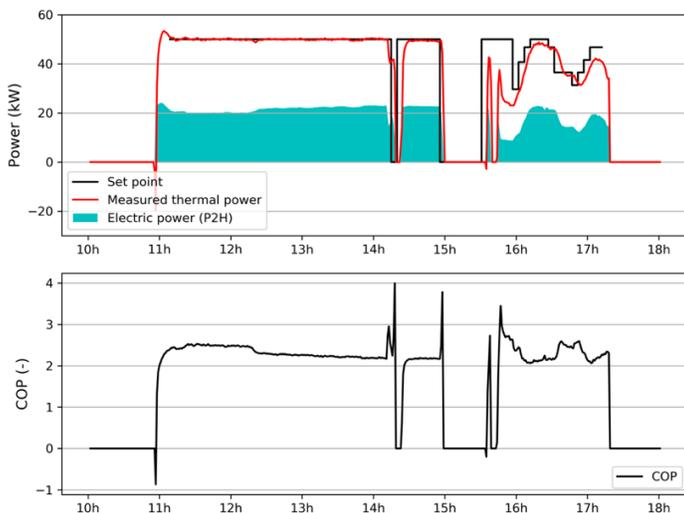
Figure 5. Profile of electric power (top), and Coefficient of Performance (bottom) during a control test
