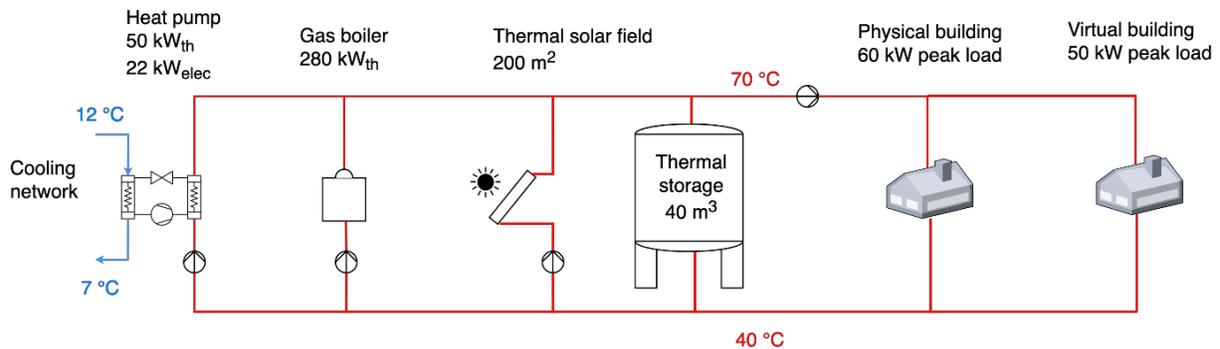
Figure 4. CEA-INES district heating network with the heat pump for P2H conversion
